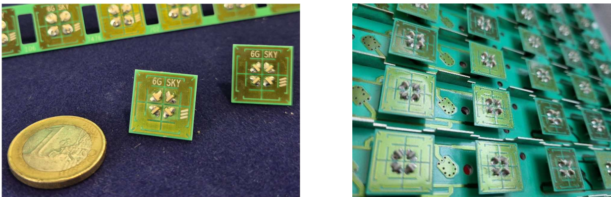
(a) Size of the radiator head (b) Radiator columns with separation walls Figure 2.9. Size comparison of a single radiator element with a euro coin (a), several radiating elements with the decoupling walls between the antenna columns (b).
