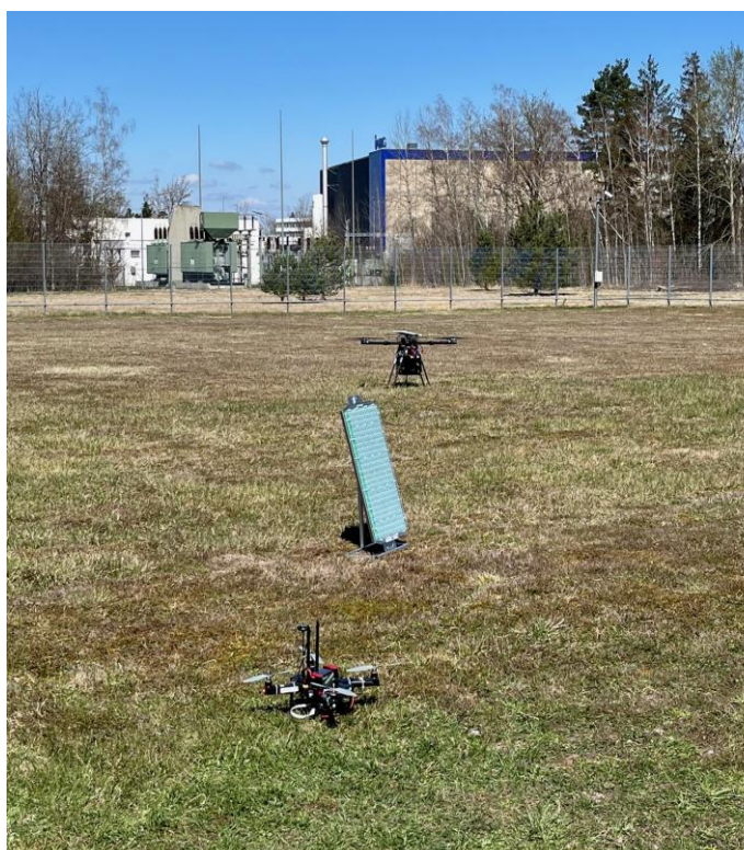
Figure 17. EAG antenna for the 6G-candidate 7GHz and the drones for the demonstrations
