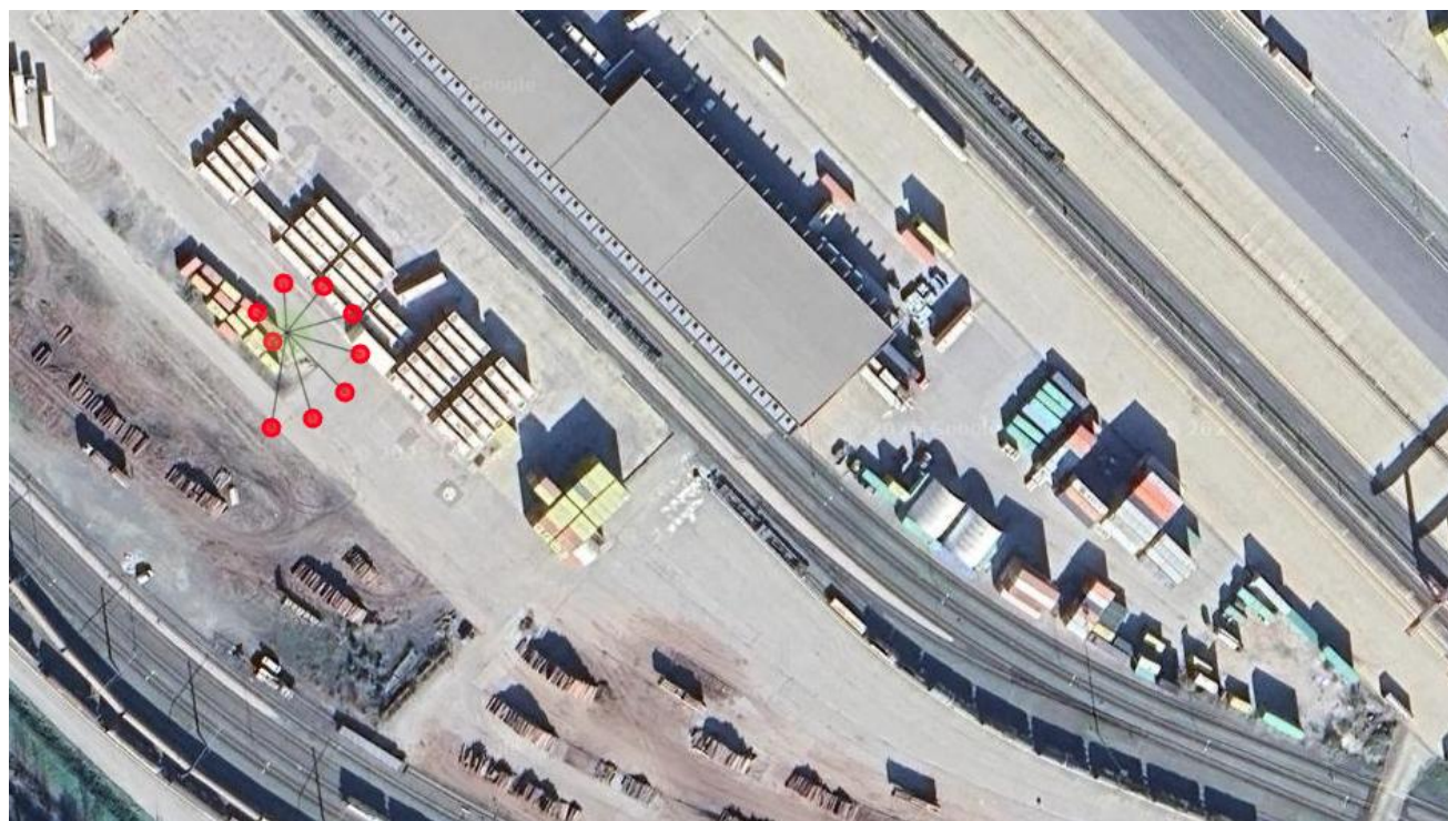
Figure 36. Overview image of the container yard with matched container IDs from the first flight. The red dots, representing GPS locations, are fanned out due to overlapping coordinates where the matching lines intersect. Note: The first flight was a test flight and only stack A was monitored
