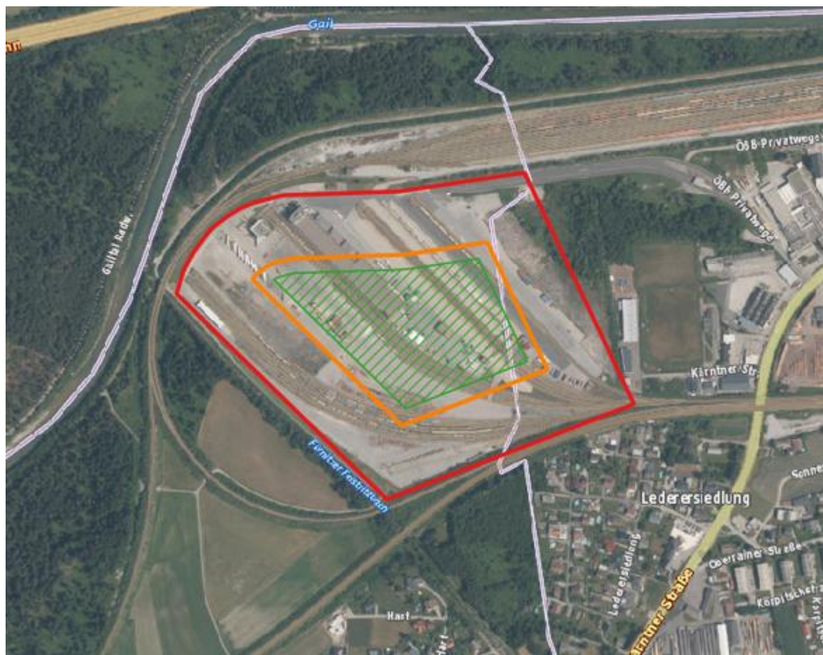
Figure 24. Reduced mission area with safety margin to reduce the ground risk
