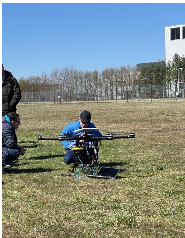
Figure 16. Preparation of the drone with multi-connectivity solutions (Wi-Fi-mesh, 5G and NTN terminals)
