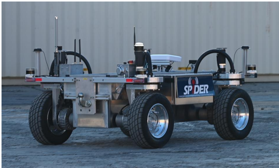
Figure 44. The SPIDER unmanned ground vehicle with the mounted mesh device (white box in the middle)
