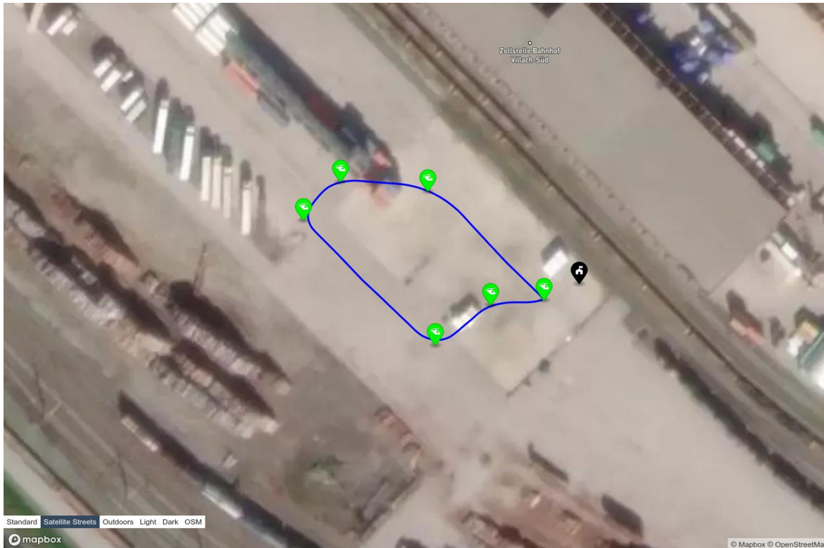
Figure 47. Setup of the use case 2 demonstration with rover path (blue), drone waypoints (green), and ground control station (black)
