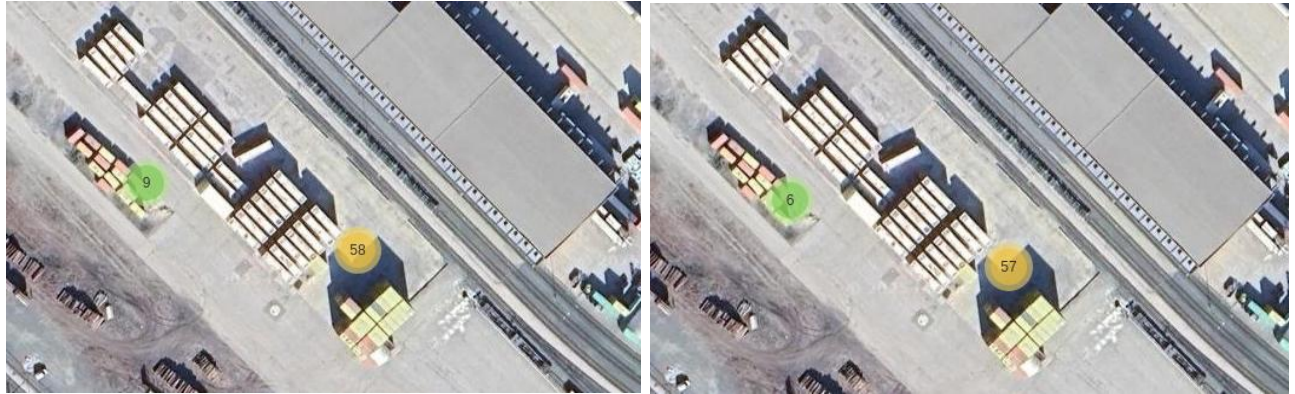
Figure 37. Container ID detection and geolocation results from the second (right) and third (left) flights for stack A (green) and stack B (yellow)
