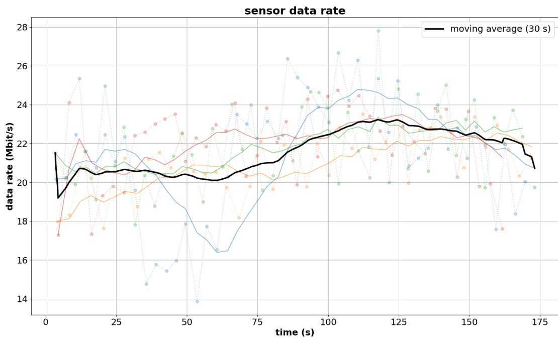
Figure 38. Measured data rate of the drone camera with 5 m spacing for different flights (colored) and averaged over all flights (black)
